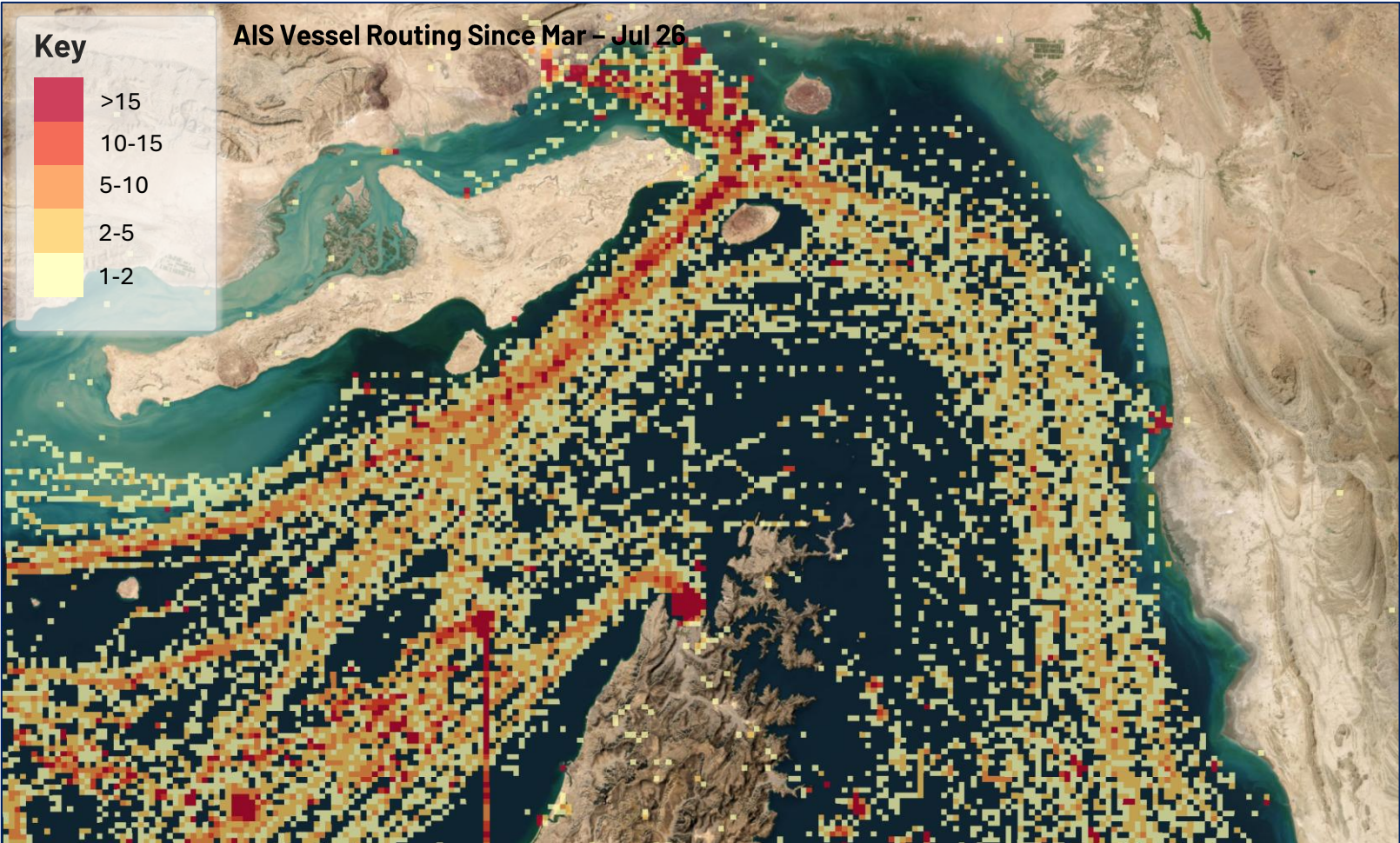
AIS-derived vessel traffic through the Strait of Hormuz (1 Mar to 31 Jul 2026). Heatmap density is based on over 100,000 AIS position reports aggregated into 1 km grid cells. Darker colours indicate higher traffic density. EMCOM silent transits are not captured.
